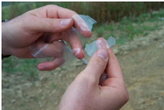
Degradable mulch film becomes brittle after desired lifetime
