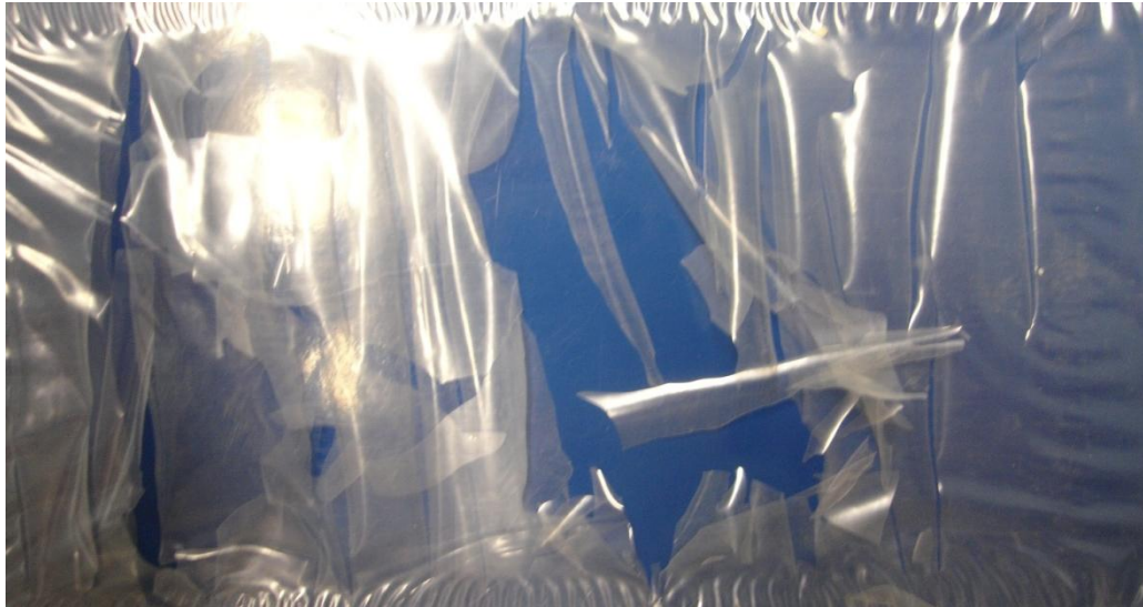
Film that has been aged 768h under accelerated UV weathering after the film has been agitated by hand.
